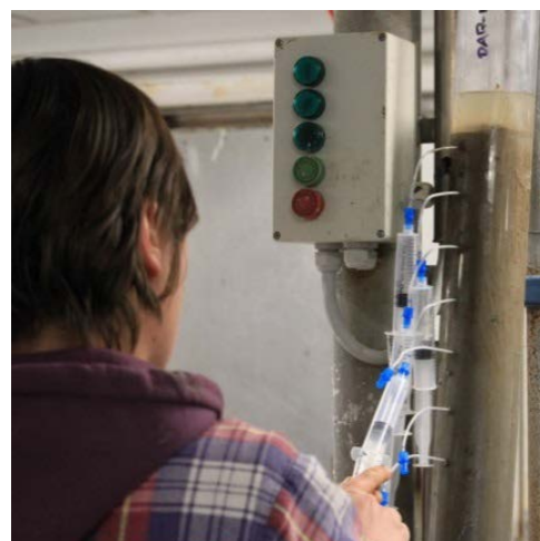
Fig. 28. Pore water subsampling from a predrilled Rumohr core into 20 mL syringes through Rhizon filters by applying vacuum. Photo: C. Scholze.
