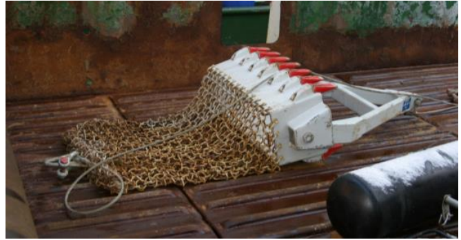
Fig. 25. The dredge, used on the NorthGreen2017 expedition. Photo by the crew of RV Dana
