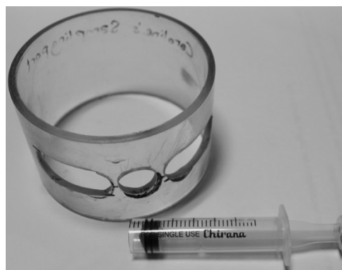
Fig. 27. Sampling port and syringe for subsampling of solid material. The Rumohr lot is extruded into the sampling port and all samples can be taken at the exact same depth. Photo by C. Scholze.
