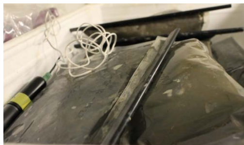
Fig. 29. Subsamples in gastight bags with a temperature logger stored in the cold room. Photo by C. Scholze.
