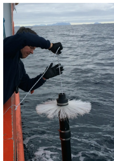
Fig. 8. Deployment of VMP-250 turbulence profiler (Photo by Søren Rysgaard)
