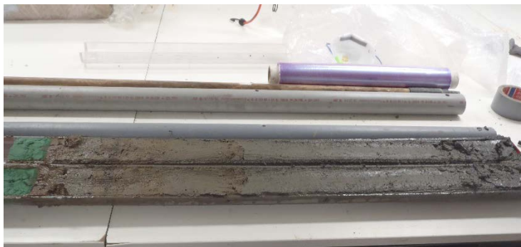
Fig. 15. To investigate the long-term response of indicator species to environmental changes, we have kept 5 Rumohr cores intact and sealed for isolating and germinating living resting cells of diatoms and dinoflagellates from dated sediment layers for time-series experiments. Other Rumohr cores were split and subsampled on board as shown here. Photo: Marianne Ellegaard.
