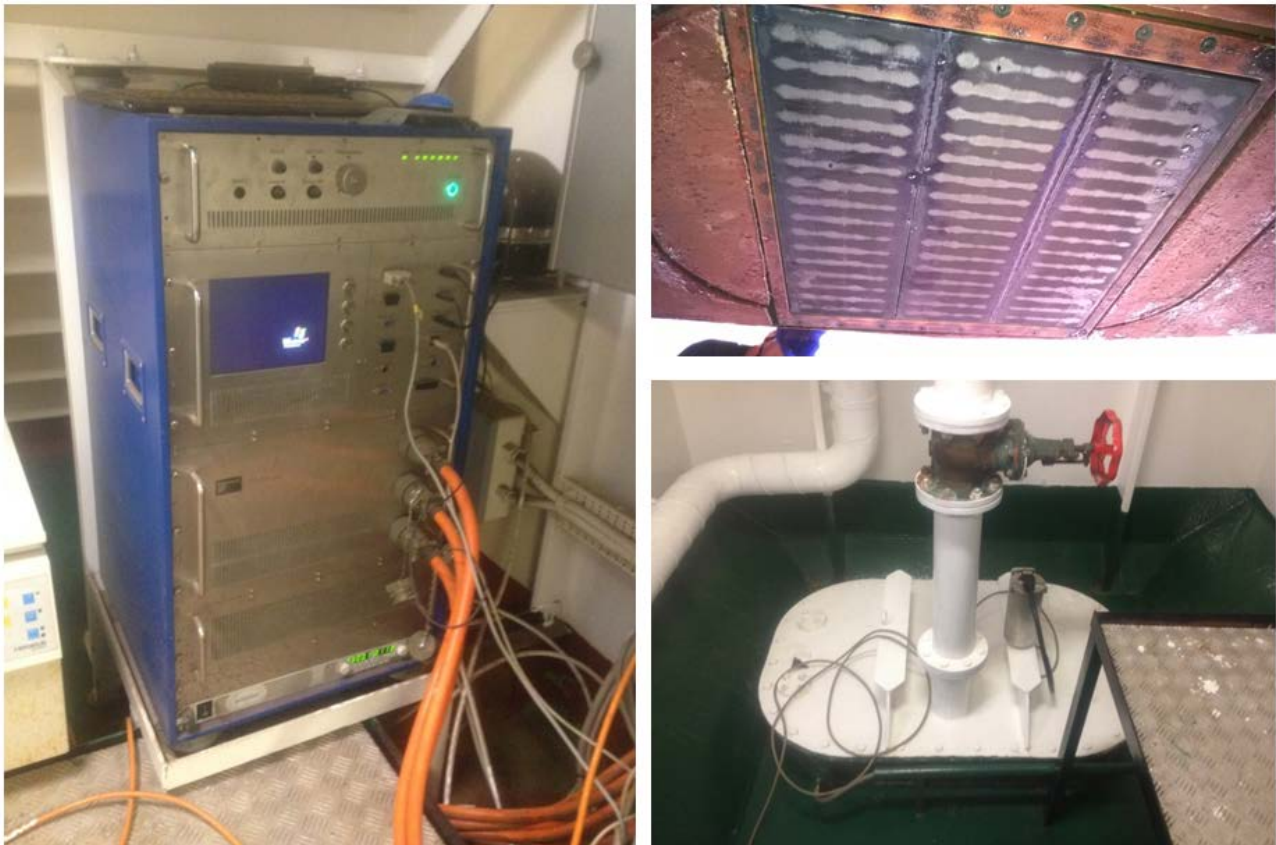
Fig. 17. Permanently installed Innomar SES-2000 Deep subbottom profiler at RV Dana. Left: transceiver unit. Right top: transducer viewed from below. The transducer transmits and receives the signal (ping). Right bottom: view at the hull mounted (moon pool installation) transducer from above (below white deck). The motion sensor (unfortunately not working) recording heave, pitch and roll variations for the SES-200 Deep instrument can be seen on top of the white deck. Photos: Katrine Juul Andresen (left) and Christian Petersen (right, both).
