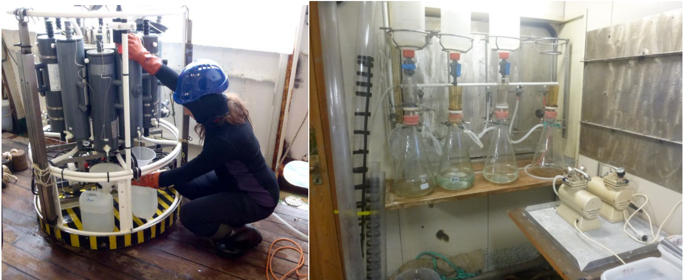
Fig. 14. Left: Water was collected during CTD casts from selected depths (surface, DCM, and bottom) and Right: immediately filtered through GF/F filters (10l per depth). A sub-sample of 250ml of water from each depth was Lugol's fixed for taxonomic determination of the plankton after the cruise. Photos: Marianne Ellegaard (Left) and Karen Gariboldi (Right).
