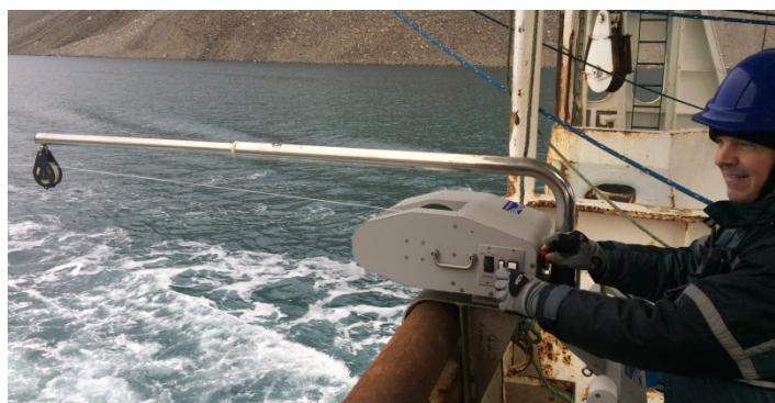
Fig. 9. Deployment of Underway CTD from the aft. Photo: Søren Rysgaard.
